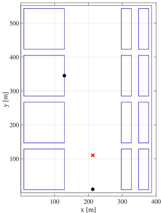
Fig. 2: Illustration of the deployment scenario considered in this paper for assessing the performance of the proposed 2-stage EKF. We have modified the Madrid grid in order to have a larger open area between BSs (black dots) and UE (red cross). The radio channel between UE and BSs is according to the METIS ray-tracing channel model [18].
