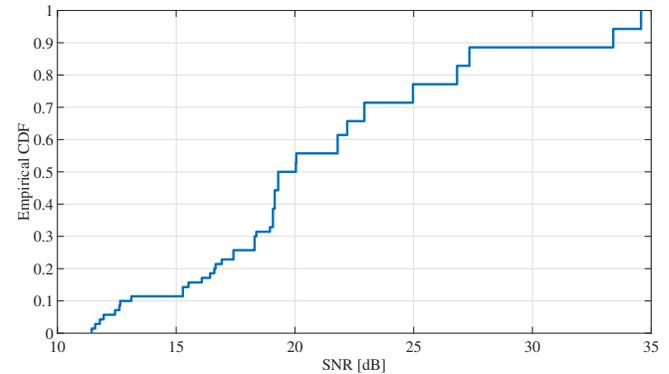
Fig. 6: Empirical CDF of received SNR at the UE, after gain from transmit/receive beams, for the 16 beams considered for reporting.
