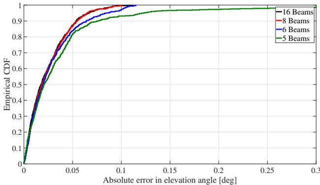
Fig. 4: Empirical CDF of elevation-angle error obtained using the proposed EKF for a varying number of feedback BRSRP measurements. Increasing the number of feedback beams improves the accuracy only slightly. This is due to the high directivity of the employed transmit beams.
