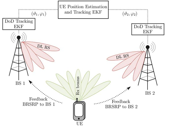
Fig. 1: Illustration of the UE positioning approach considered in this paper. In particular, UEs feedback RSRP measurements obtained from DL RSs and transmitted across multiple BS beams. Only angles are used for positioning purposes. A single BS suffices in determining the 2D position of a UE given that its height is known. For 3D positioning at least two BSs are needed.
