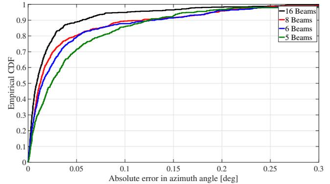
Fig. 5: Empirical CDF of azimuth-angle error obtained using the proposed EKF for a varying number of feedback BRSRP measurements. Increasing the number of feedback beams improves the accuracy only slightly. This is due to the high directivity of the employed transmit beams.
