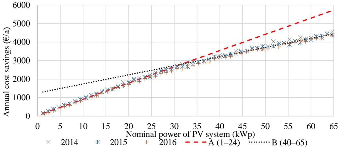
Fig. 7. Cost simulation for apartment building using various sizes of PV system (Fig. 1). Line *A* is the result of a linear regression performed on data points between 1–24 kWp nominal power of PV system and line *B* that of between 40–65 kWp.
