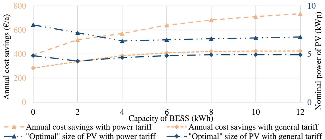
Fig. 12. Sizing of the PV system using various sizes of BESS.
