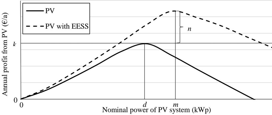
Fig. 4. The basic principle of PV sizing.
