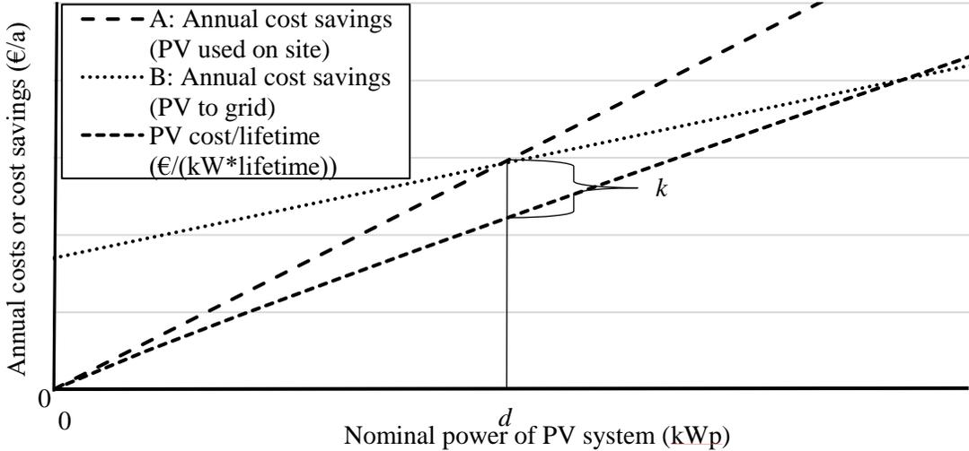
Fig. 3. The basic principle of PV sizing.
