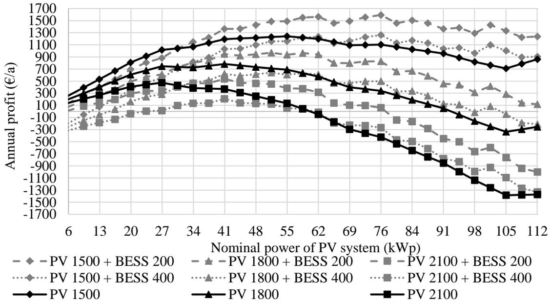
Fig. 10. Annual profit from various sizes of PV system both with and without 25 kWh BESS, when the energy community model with the low-voltage power tariff is applied. Three alternatives for the PV investment price (1500, 1800, and 2100 €/kWp) and two alternatives for the BESS investment price (200 and 400 €/kWh) are presented.
