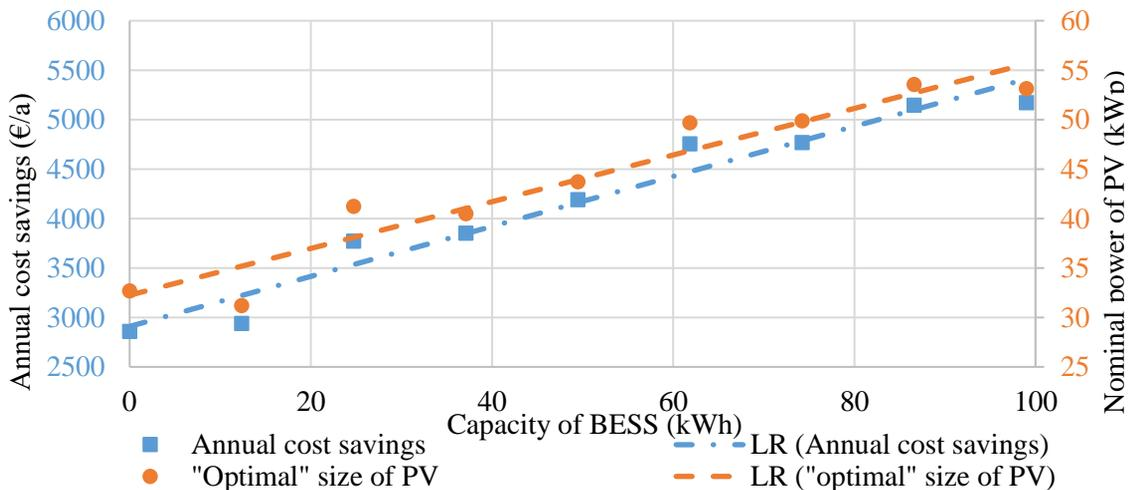
Fig. 8. Effect of BESS on annual cost savings from PV and “optimal” size of PV.
