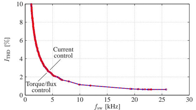
Fig. 5: Trade-off between current THD  $I_{\text{THD}}$  and switching frequency  $f_{\text{sw}}$  for current FCS-MPC (solid, blue line), and torque/flux FCS-MPC (dashed, red line). The individual simulations are shown as squares (current control), and circles (torque/flux control).
