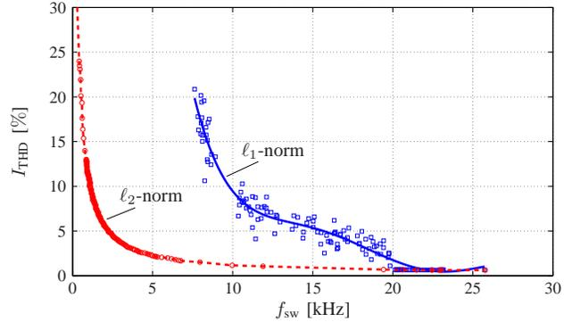
Fig. 4: Trade-off curves for the stage cost (9) with  $\ell_1$ - and  $\ell_2$ -norm. The current THD  $I_{\text{THD}}$  is shown for the achievable range of switching frequencies  $f_{\text{sw}}$ . The solid (blue) and dashed (red) lines are polynomial approximations of the individual simulation results. The individual simulations are indicated by squares and circles for current FCS-MPC based on the  $\ell_1$ - and  $\ell_2$ -norm, respectively.
