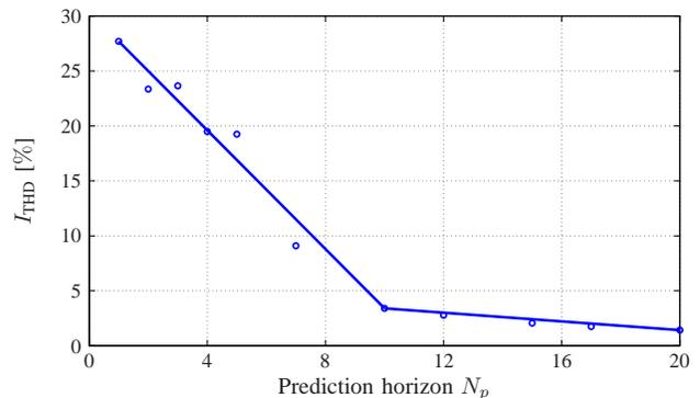
Fig. 10: Stator current THD  $I_{\text{THD}}$  of a third-order drive system as a function of the prediction horizon  $N_p$  at a switching frequency of  $f_{\text{sw}} \approx 3$  kHz. Individual simulations are shown as circles.
