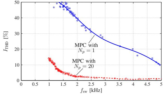
Fig. 9: Third-order (two-level inverter with an  $LC$  filter and IM) system: trade-off between stator current THD  $I_{\text{THD}}$  and switching frequency  $f_{\text{sw}}$  for FCS-MPC with  $N_p = 1$  (solid, blue line), and FCS-MPC with  $N_p = 20$  (dashed, red line). The individual simulations are shown as squares (MPC with  $N_p = 1$ ), and circles (MPC with  $N_p = 20$ ).
