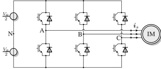
Fig. 15: Two-level inverter driving an induction machine.
