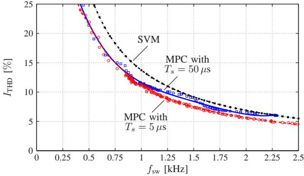
Fig. 7: Trade-off between current THD  $I_{\text{THD}}$  and switching frequency  $f_{\text{sw}}$  for FCS-MPC with  $T_s = 50 \mu\text{s}$  (solid, blue line), FCS-MPC with  $T_s = 5 \mu\text{s}$  (dashed, red line), and SVM (dash-dotted, black line). The individual simulations are shown as squares (MPC with  $T_s = 50 \mu\text{s}$ ), circles (MPC with  $T_s = 5 \mu\text{s}$ ), and asterisks (SVM).
