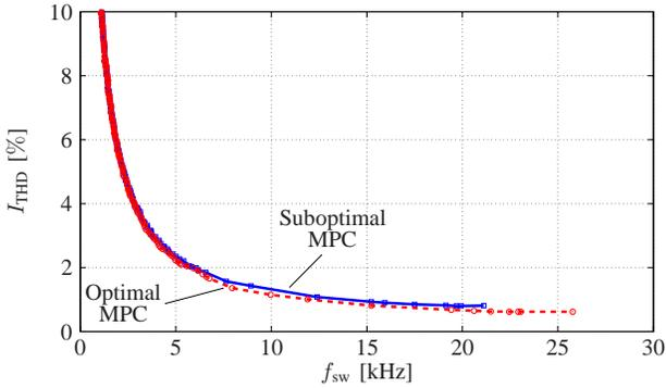
Fig. 13: Trade-off between current THD  $I_{\text{THD}}$  and switching frequency  $f_{\text{sw}}$  for suboptimal MPC via direct rounding (solid, blue line), and optimal FCS-MPC (dashed, red line). The individual simulations are shown as squares (suboptimal MPC), and circles (optimal MPC).
