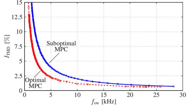
Fig. 11: Trade-off between current THD  $I_{THD}$  and switching frequency  $f_{sw}$  for suboptimal (solid, blue line), and optimal (dashed, red line) torque/flux FCS-MPC. The individual simulations are shown as squares (suboptimal FCS-MPC), and circles (optimal FCS-MPC).
