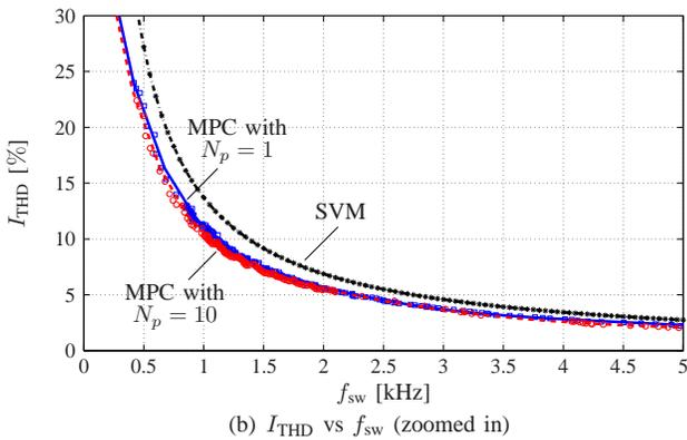
Fig. 8: First-order (two-level drive) system: trade-off between current THD  $I_{\text{THD}}$  and switching frequency  $f_{\text{sw}}$  for FCS-MPC with  $N_p = 1$  (solid, blue line), FCS-MPC with  $N_p = 10$  (dashed, red line), and SVM (dash-dotted, black line). The individual simulations are shown as squares (MPC with  $N_p = 1$ ), circles (MPC with  $N_p = 10$ ), and asterisks (SVM).
