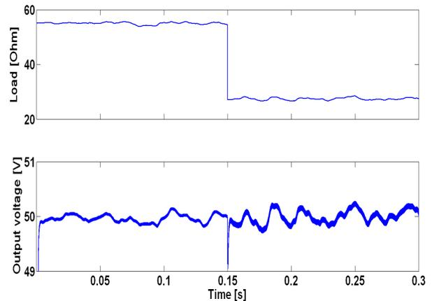
Fig. 6. Load resistance variations and corresponding output voltage
