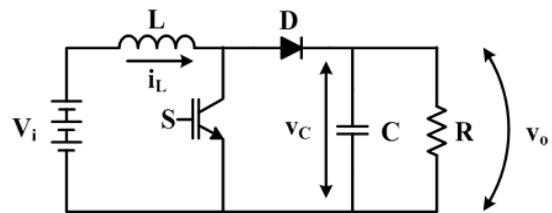
Figure 1. DC-DC boost converter topology
