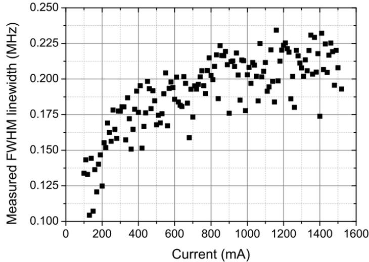
**Figure 4. Measured linewidth from 100 mA to 1.5A.**
