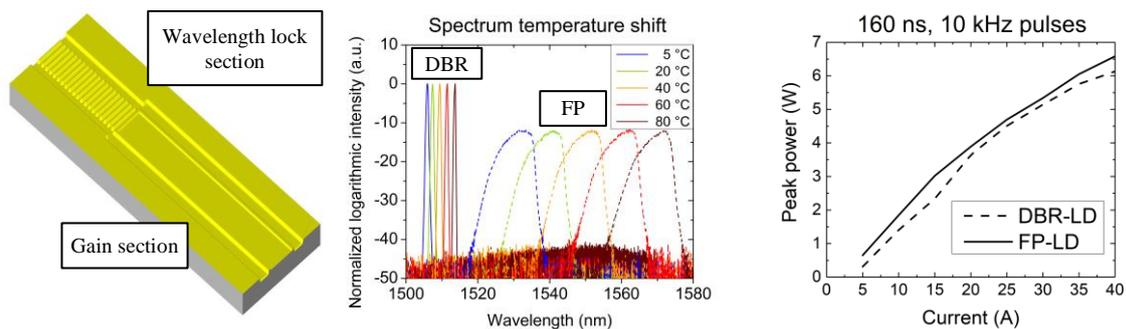
**Fig. 1** Left panel (a): schematic illustration of the DBR laser. Center panel (b): spectral characteristics of a wavelength stabilized DBR laser and non-stabilized (FP) laser overlaid on same graph. Right panel (c): comparison of LI-characteristics.
