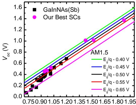
Fig. 2.  $V_{oc}$  values for Band gap (eV) lattice-matched solar cells with different junction bandgap values determined using one sun AM1.5 (1000 W/m<sup>2</sup>) illumination.
