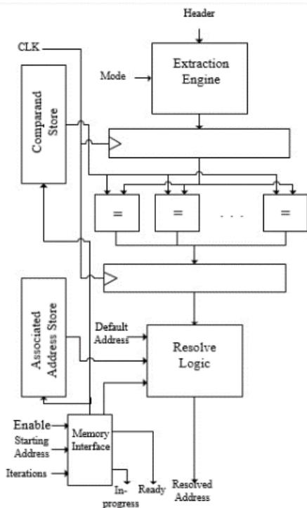
Fig. 5. The internal components of the NHRU
