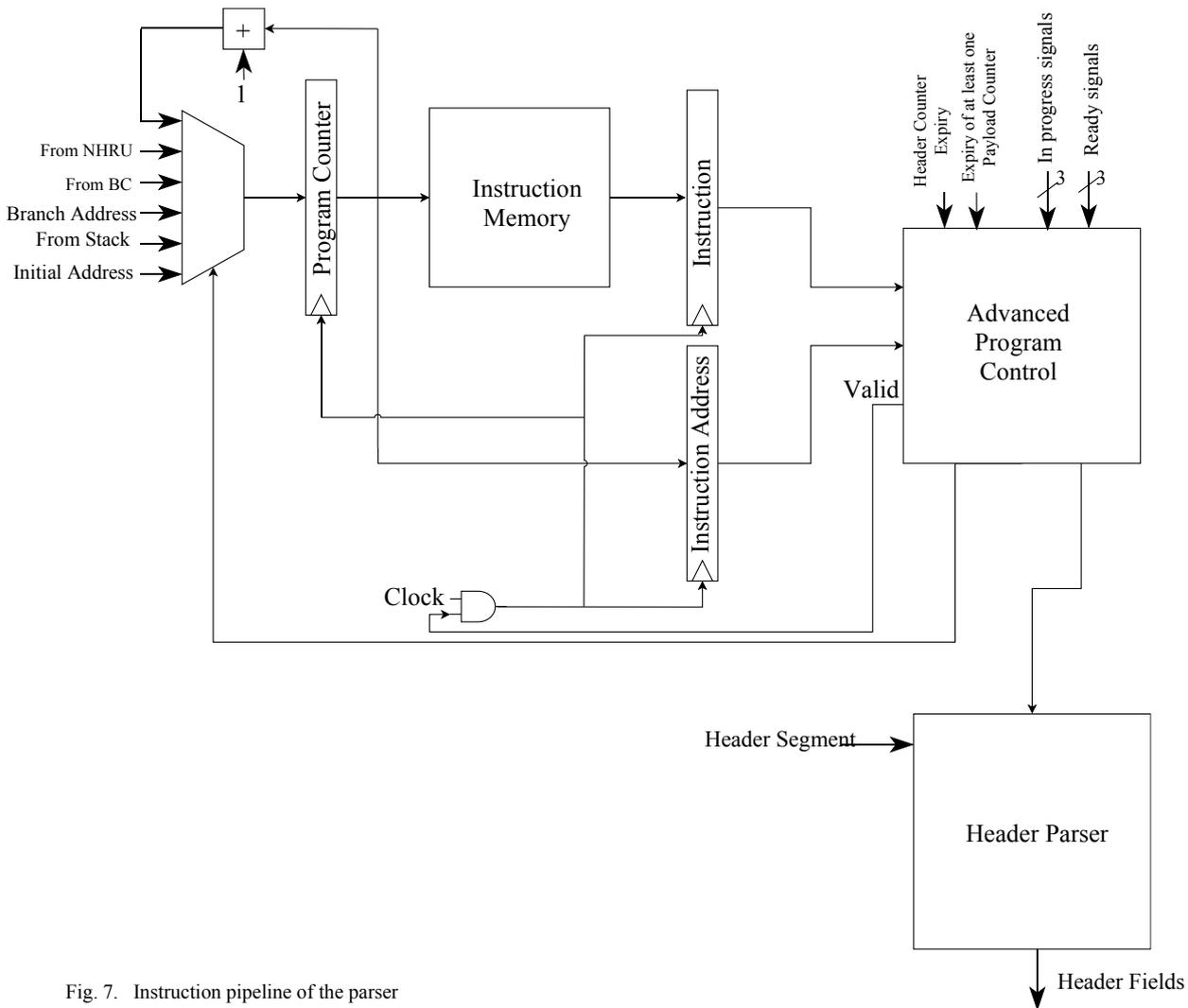
Fig. 7. Instruction pipeline of the parser
