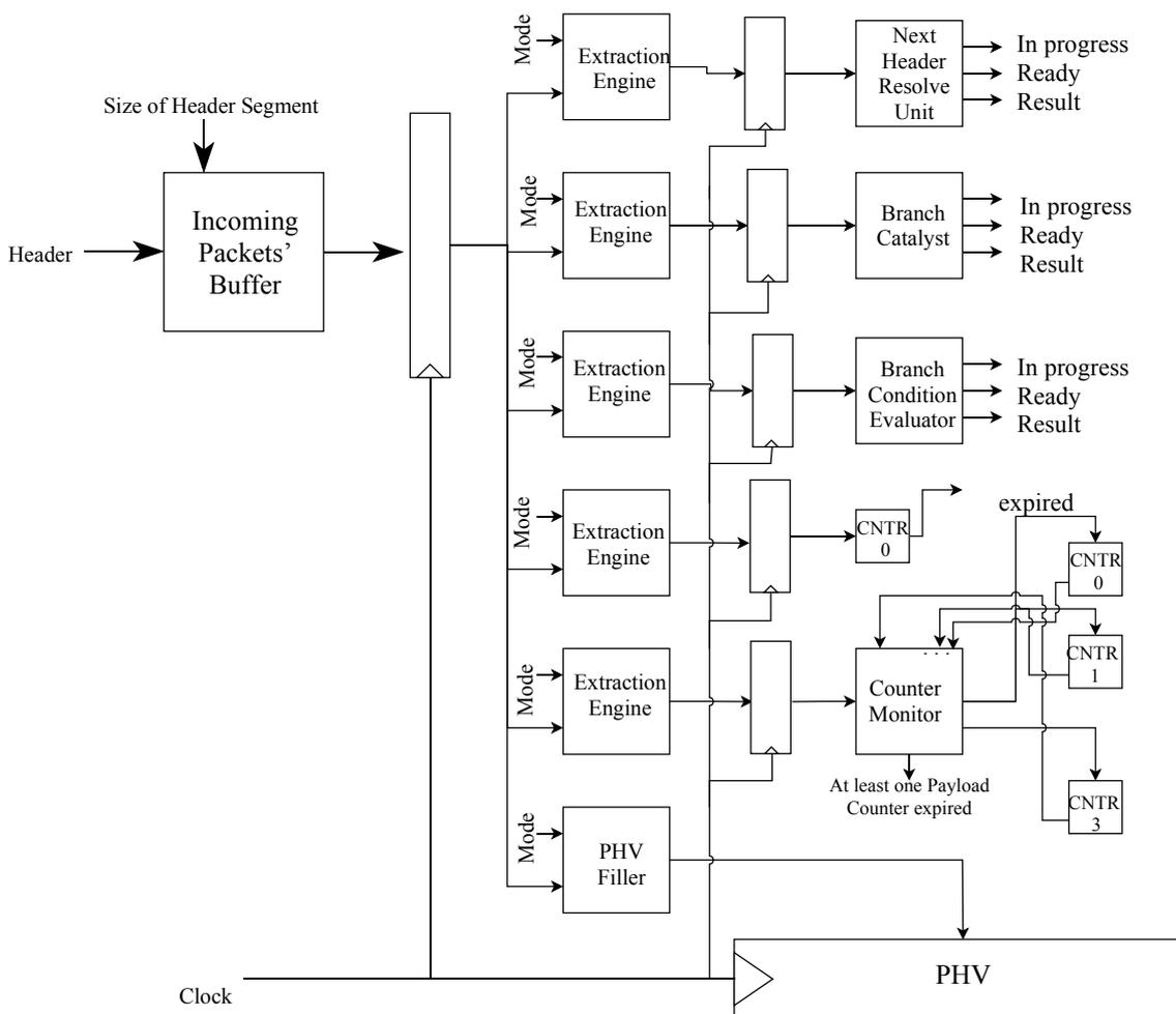
Fig. 6. Internals of the explicitly parallel header parser
