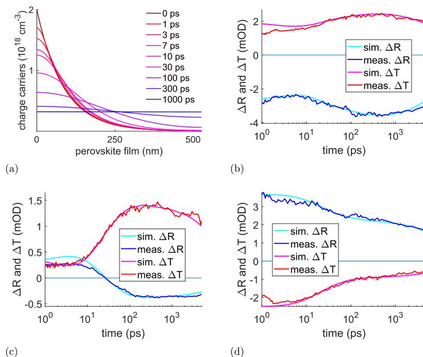
**Figure 2.** Simulated (a) charge carrier density distributions and (b–d) resulting transient reflectance and transmittance signals at wavelengths 880, 936, and 1040 nm, respectively. Surface roughness was included in this simulation; the diffusion constant was  $1.64 \text{ cm}^2 \text{ s}^{-1}$ , and the lifetime was 14.7 ns.  $\Delta T$  was multiplied by 4 for clarity.
