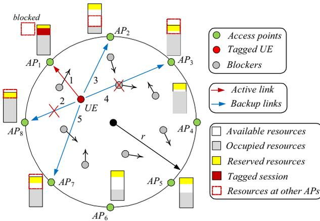
Fig. 1. Considered deployment: multi-connectivity and guard bandwidth.
