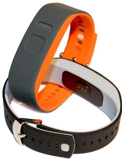
Figure 1. PulseOn optical wrist-worn heart rate monitor used in the study.
