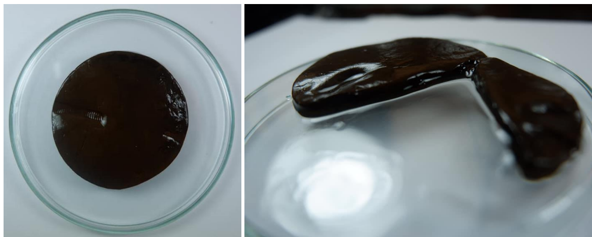
Fig. S1. Optical images the BC hydrogel after the incorporation of \text{MnFe}_2\text{O}_4 nanoparticles by the co-precipitation method. The image on the right shows the cross-section of the hydrogel with the nanoparticles dispersed homogeneously throughout the samples.
