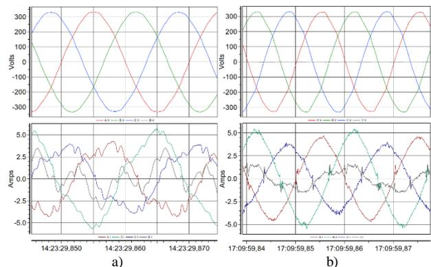
Figure 3. Phase voltage and current waveforms from FTLs with magnetic ballast (a) and electronic ballast (b). L1 is red, L2 is green, L3 is blue and grey is neutral.
