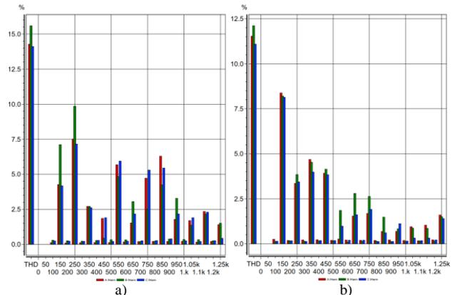
**Figure 6.** Measured current THD of LED tubes with capacitors (a) and without capacitors (b). L1 is red, L2 is green, and L3 is blue.
