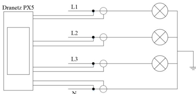
Figure 2. Measurement setup.
