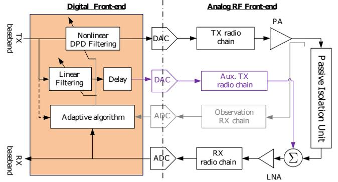
Fig. 1. The proposed architecture of the simultaneous transmit-receive radio transceiver, employing a digital pre-distorter to linearize the TX PA and active RF canceller for suppressing the TX leakage signal.
