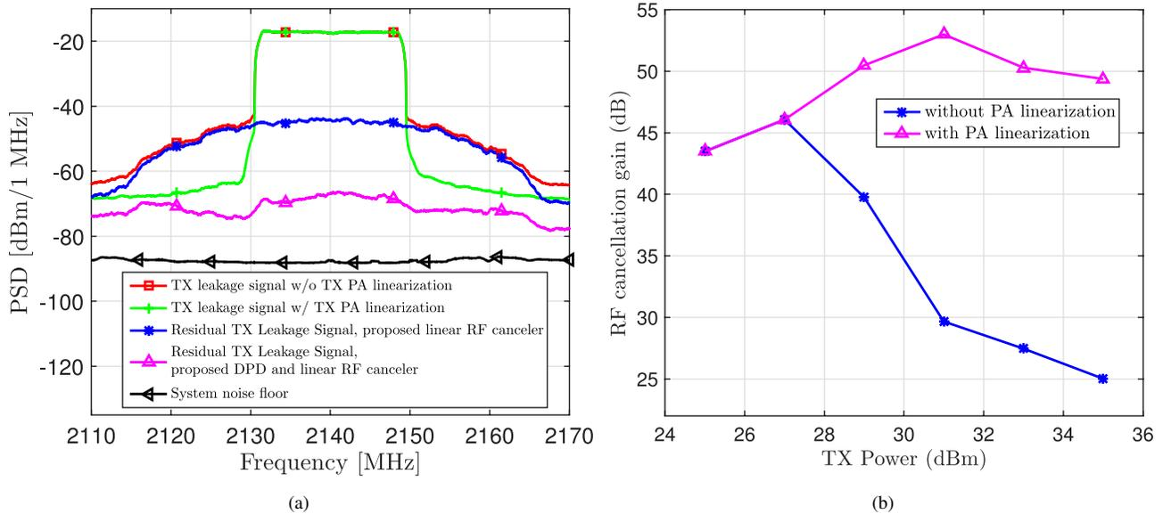
Fig. 3. The performance results of the proposed technique at +35 dBm TX power and with 40 dB passive isolation. TX signal bandwidth is 20 MHz. (a) measured signal power spectral density curves referred to LNA input with and without active RF cancellation ; (c) measured RF cancellation gain against different TX power with and without TX PA linearization.
