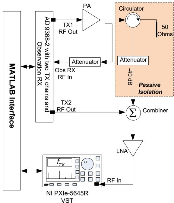
Fig. 2. Block diagram of the RF measurement setup used for evaluating the performance of the proposed technique.
