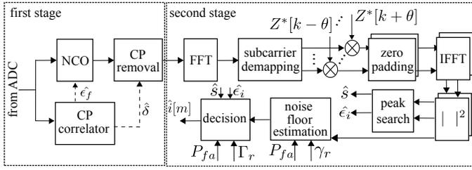
Fig. 4. Block diagram of main components of WRx.
