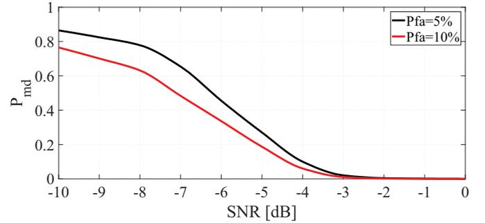
Fig. 6. Misdetection rate as a function of SNR, at fixed false alarm rates.
