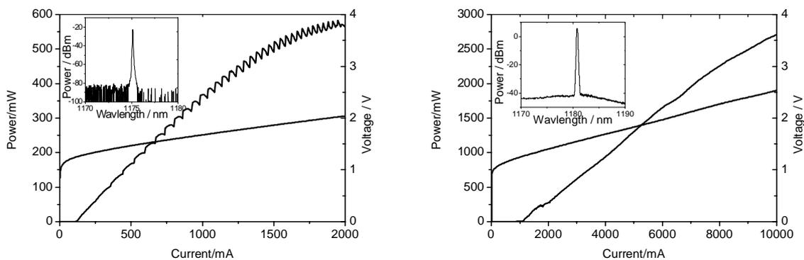
**Fig. 1** Left panel: ILV for non-tapered DBR-LD in CW at room temperature. Inset shows measured spectrum at 1.5A. Right panel: LIV for tapered DBR-LD at room temperature. Current is swept in tapered section. Inset shows spectrum at 6A tapered section operation current. In both measurements with tapered DBR-LD ridge waveguide section current is fixed to 250mA.
