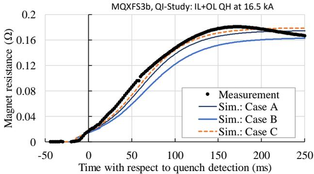
Figure 7: Measured magnet resistance in MQXFS3b after OL and IL heater activation compared with different simulation scenarios.
