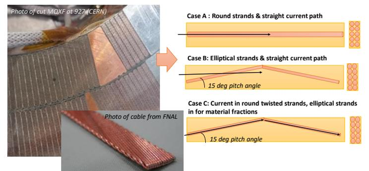
Figure 5: Three cases how the current flow in quenched cable can be simulated.
