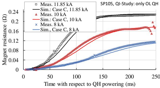
Figure 10: Current decay after OL heater powering in 11 T SP105 and comparison with simulation.
