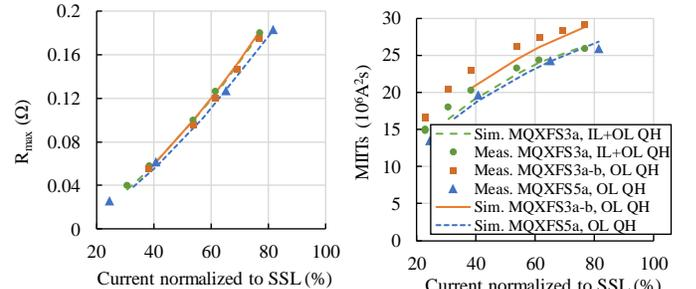
Figure 9: Summary of measured and simulated final magnet resistances and MIITs from MQXFS3 and MQXFS5 models. The magnet current is normalized to the short sample limit (21.4 kA).
