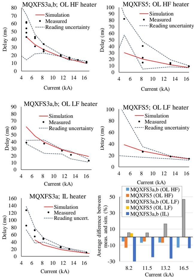
Figure 3: Summary of heater delays in MQXFS models, and the difference between simulation and measurement. The maximum reading uncertainty associated with the measurement at each current is shown.
