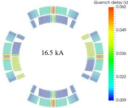
Figure 6: Simulated heater delays in MQXFS3 at nominal current when two inner layer heater strips are disconnected.
