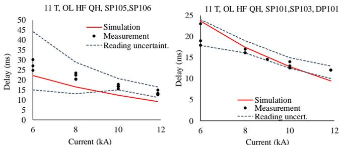
Figure 4: Summary of heater delays in 11 T models with impregnated heaters.
