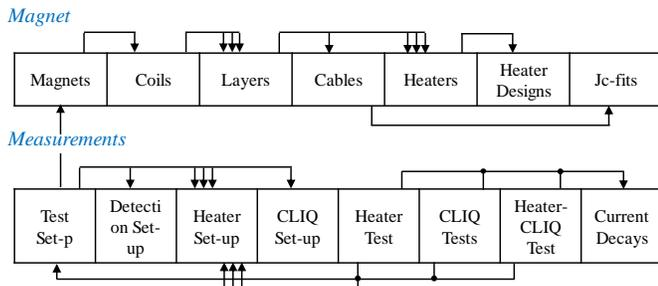
Figure 1: A schematic of the database structure. Data is divided into two categories: *Magnet*, for magnet design parameters, and *Measurements*, to describe the test set-up, and the results from quench protection tests. The arrows indicate links between tables. A triple-arrow indicates that each item can be connected to several items in the target table, for example a coil can be connected to several layers.
