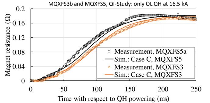
Figure 8: Measured and computed coil resistance in MQXFS3b and MQXFS5 when OL heaters activated at nominal current. The heater peak power is 200 W/cm<sup>2</sup> in MQXFS5 and 110 W/cm<sup>2</sup> in MQXFS3 models.
