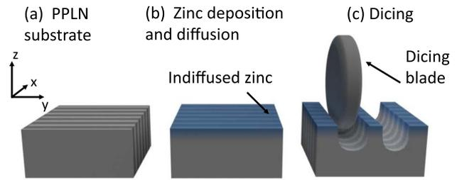
**Fig. 1.** Fabrication process flow of the zinc-indiffused PPLN waveguides.
