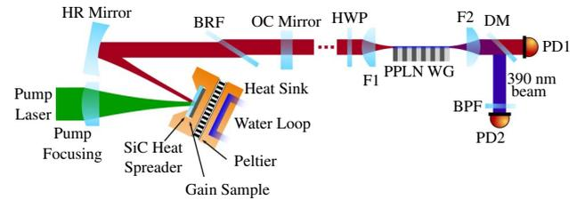
**Fig. 4.** VECSEL cavity configuration and the position of the PPLN waveguide in the setup, which is utilized as an extra-cavity component.
