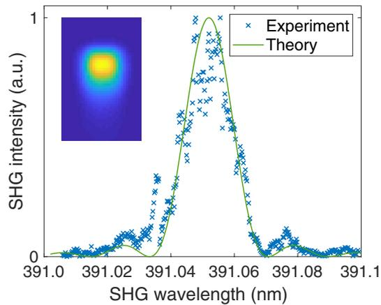
**Fig. 3.** PPLN waveguide phase-matching spectrum characterization performed through lock-in amplification detection at room temperature. Inset shows the output profile of the 780 nm mode propagating in this waveguide.
