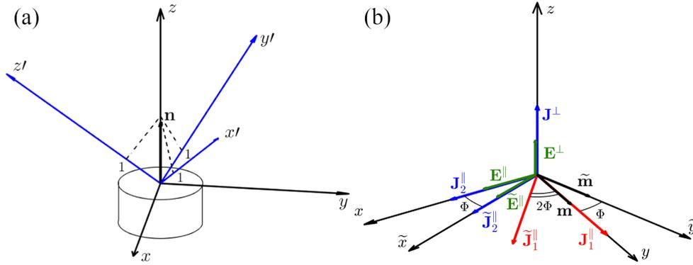
**Figure 1.** (a) Crystalline and laboratory coordinate systems. The disk-shaped particle is grown along the (111) normal  $\mathbf{n}$ . (b) Scheme of the nonlinear source rotation in the case of single-mode approximation. The FW field inside the particle is assumed to be described by the magnetic dipole mode with magnetic moment  $\mathbf{m}$ .
