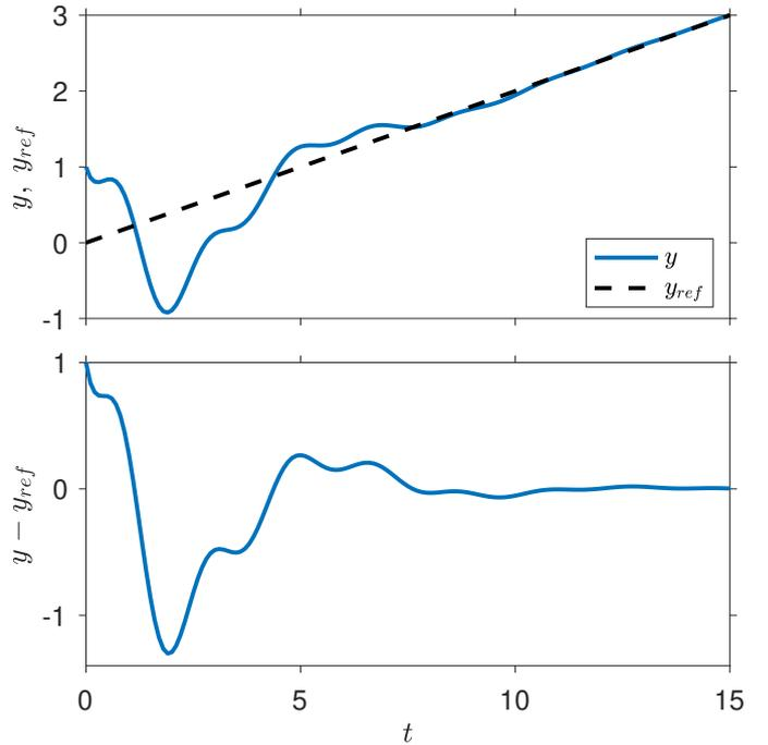
Fig. 1. Above: the reference signal  $y_{ref}$  and the output  $y$ . Below: the regulation error  $e = y - y_{ref}$ .
