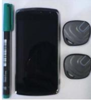
Figure 2. BeSpoon phone and six tags equipped with UWB.
