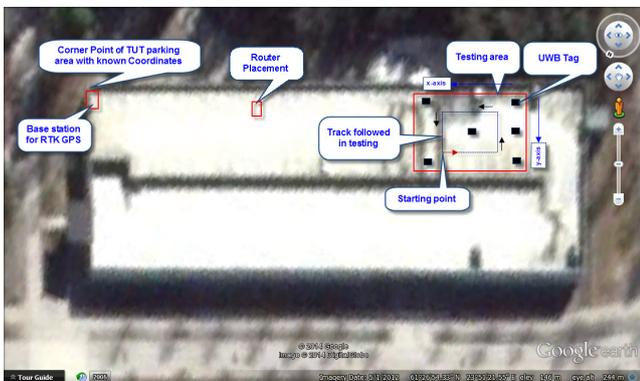
Figure 5. Google Earth view of testing setup. Parking is approximately 100 m long and 30 m wide.
