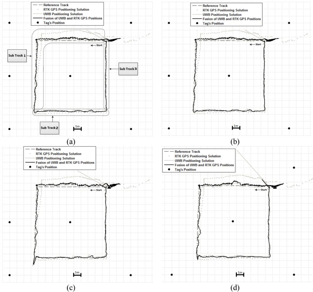
Figure 6. (a) Result with 6 UWB tags and track is divided into three sub tracks (b) Result with cycle slip (simulated) when 6 UWB tags are used (c) Result with 4 UWB tags second scenario (d) Result with 4 UWB tags third scenario.
