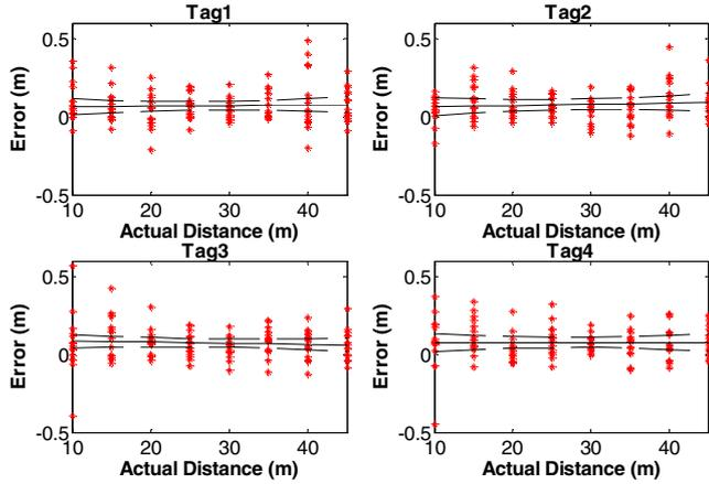
Figure 3. Dynamic line-of-sight error measurement (\*), linear regression line (continuous line) and 95% credibility interval limits (dashed line).
