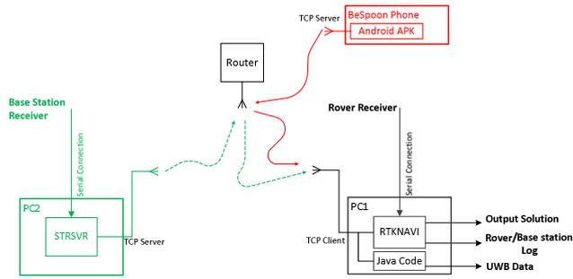
Figure 4. UWB and RTK GPS fusion configuration in our measurements.
