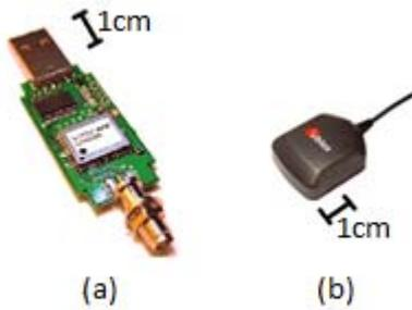
Figure 1. (a) Yuan10 USB receiver (b) ANN-MS u-blox active GPS antenna
