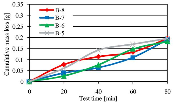
Figure 9. Cumulative mass loss results from the sample rotation test for rubber A (on the left) and for rubber B (on the right). The sample levels and the slurry were changed after each 20 minute run.
