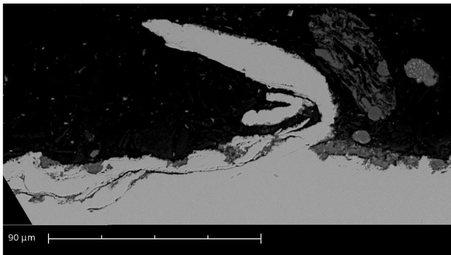
*Figure 11. Wear surface cross-section of an AISI 316 sample.*
