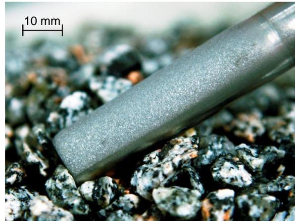
Figure 3. Round AISI 316 sample with granite gravel.
