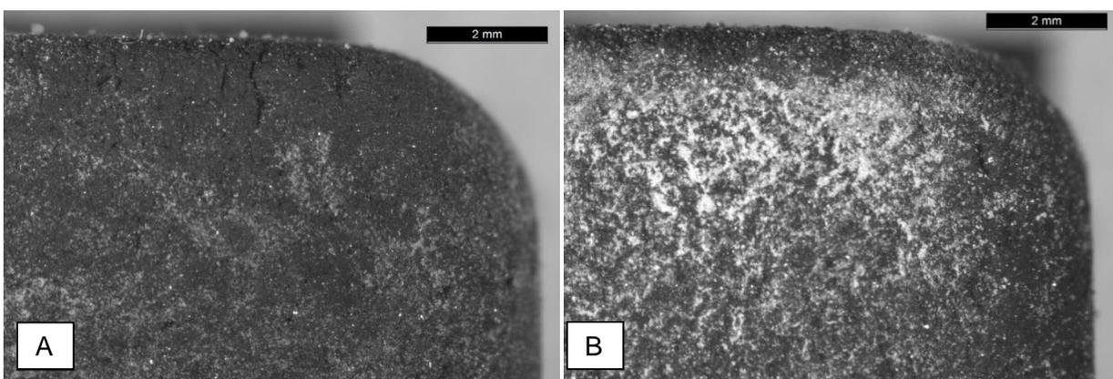
*Figure 12. Wear surfaces from the leading edge of the tested rubbers. A) In rubber sample A, surface cracks on the edge are clearly visible and the tip is intensively rounded. B) In rubber sample B, no visible cracks on the edge can be observed and the rounding of the tip is much smaller.*
