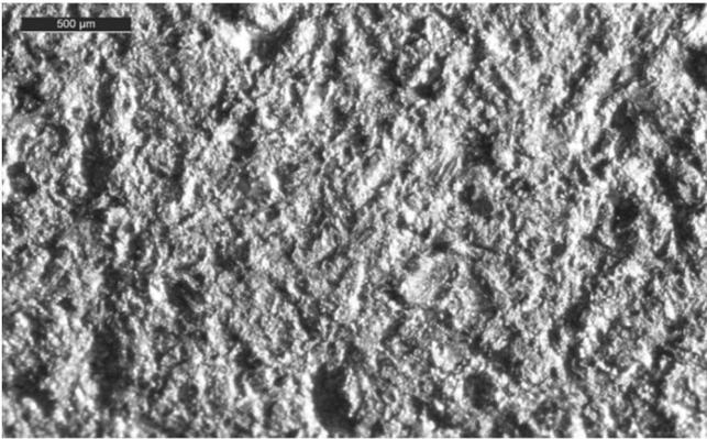
Figure 11 presents a scanning electron microscope image of the wear surface cross-section. The cross-section is taken 3.5 cm behind the sample tip, where the tip rounding ends. Embedding of the abrasive particles, abrasive cutting of the surface, and peeling off of the deformed surface layers are all visible. Hard granite particles embed easily on the 200 HV steel surface, and sharp particles moving at high speeds produce abrasive microcutting.
