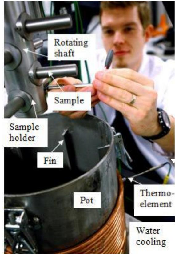
Figure 1. The pin mill type slurry-pot unit.
