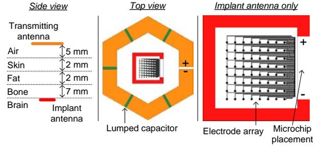
Fig. 2 Simulation model of the wireless link.
