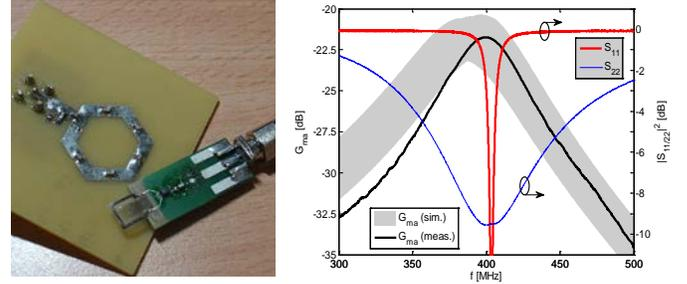
Fig. 5. Fabricated devices, the measured and simulated  $G_{ma}$  in air with the antenna separation of 2 cm, and the measured input reflection coefficients.
