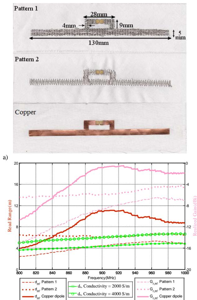
Fig. 3. (a) The upper T-matched dipole is sewed with Pattern 1, the dipole in the middle is sewed with Pattern 2, and the lowest one is a T-matched copper dipole, (b) measurement and simulation results of the dipoles shown in the picture.
