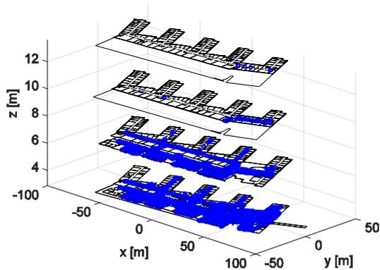
Figure 2. BLE measurements in a 4-floor university building (the position of the fingerprints is shown in blue circles).
