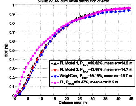
Figure 6. Distance error CDF based on WLAN 5 GHz signals.
