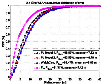
Figure 5. Distance error CDF based on WLAN 2.4 GHz signals.
