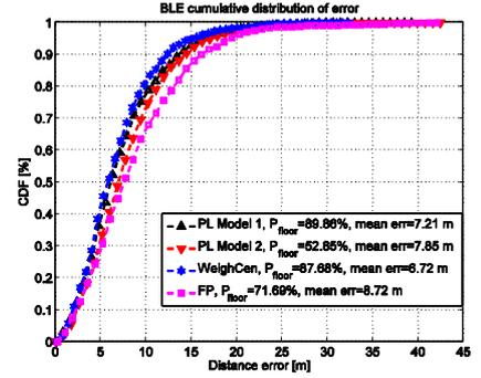
Figure 7. Distance error CDF based on BLE 2.4 GHz signals.
