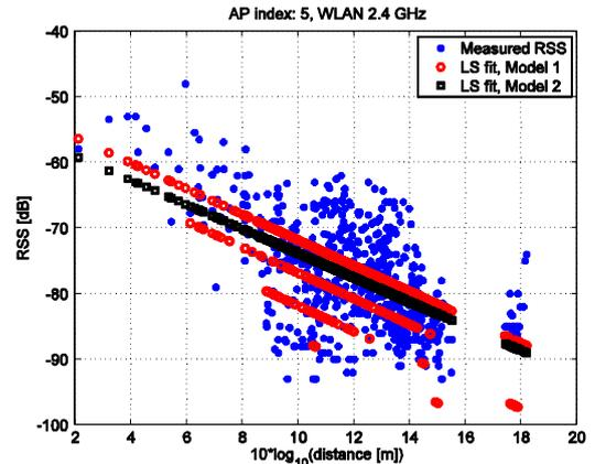
Figure 3. Example of the Least Squares fit for the two path-loss models.
