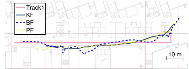
Figure 4: KF, BF and PF estimates for test track 1
