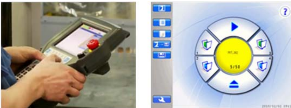
Figure 2. Comparison of interfaces of traditional teach pendant (left) and the novel player interface (right).
