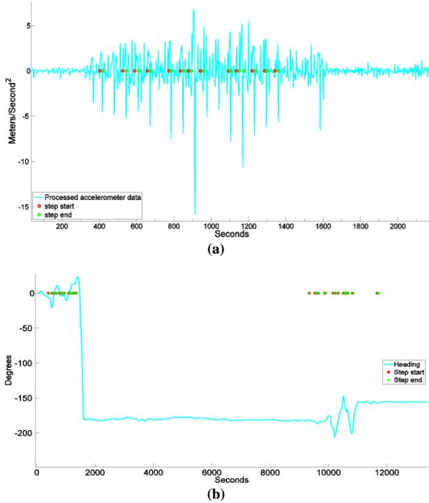
**Fig 2 (a) Processed accelerometer data representing walker motion and (b) processed gyroscope data representing walker's heading estimate. Detected steps are plotted with start and end markings for each step on both (a) and (b) plots.**
