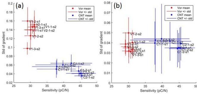
Fig. 6. Sensitivities ( $s_1 = \text{side 1}$ ,  $s_2 = \text{side 2}$ ) of the Vor-ink (V) and CNT-ink (C) sensors ( $n = 3$ ) plotted against the surface roughness parameter, i.e., standard deviation (std) of the gradient. (a) Roughness parameter based on the unfiltered y-gradient images. (b) Roughness parameter based on the low-pass filtered x-gradient images; limit wavelength  $100 \mu\text{m}$ .
