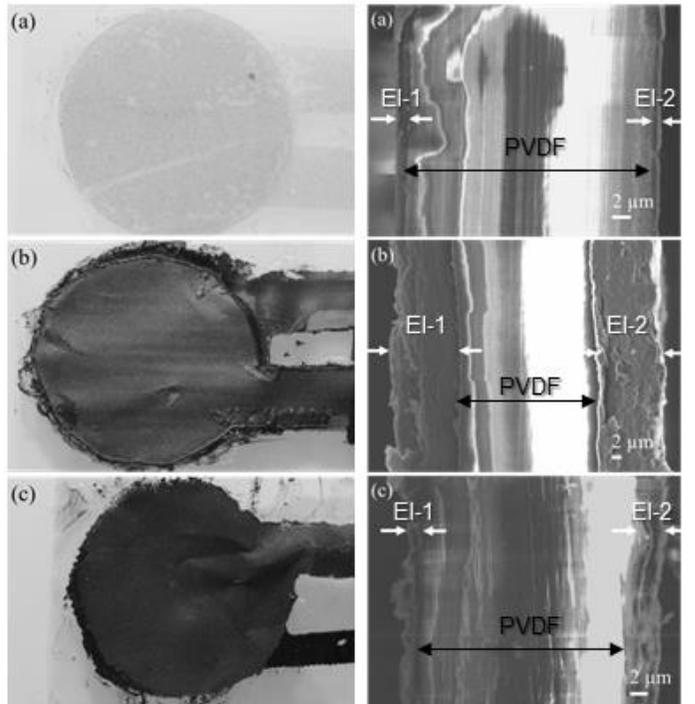
Fig. 5. Examples of the photographs and SEM images of cross-sections of PVDF sensors with a) Phene-ink (R1-1 from side 1, illumination polar angle  $\sigma = 45^\circ$ ), b) Vor-ink (R1-1 from side 1, illumination polar angle  $\sigma = 60^\circ$ ) and c) CNT-ink (R1-2 side 2, illumination polar angle  $\sigma = 75^\circ$ ) electrodes (EI-1 = electrode 1, EI-2 = electrode 2).
