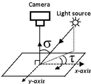
Fig. 4. Photometric stereo imaging principle. The camera was situated at polar angle  $\sigma = 0^\circ$  and the light sources were at  $\sigma = 75^\circ$ ,  $\sigma = 60^\circ$  and  $\sigma = 45^\circ$ . For each value of  $\sigma$ , the four light sources (of which one is shown) had azimuth angles ( $\tau$ )  $90^\circ$  apart from each other.
