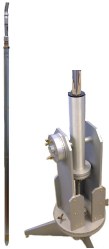
Fig. 1: Sonde instrument on the left and on the right is the jig that were used in obtaining sensor data for experiments.
