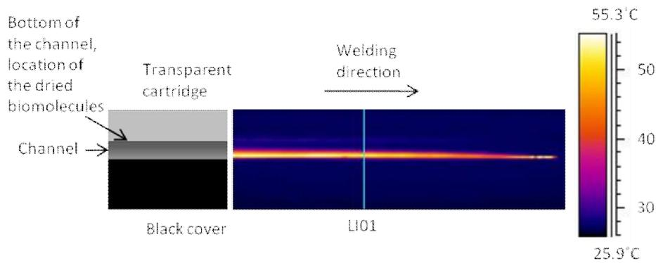
FIG. 8. Thermal image captured 0.13 seconds after the beam has passed the line LI01 using a 100 µm welding distance between the seam and the channel wall.
