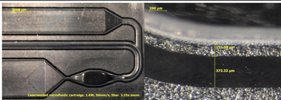
FIG. 4. Stereo microscope images from top direction of the welding seam using 3.15x and 64x zoom.
