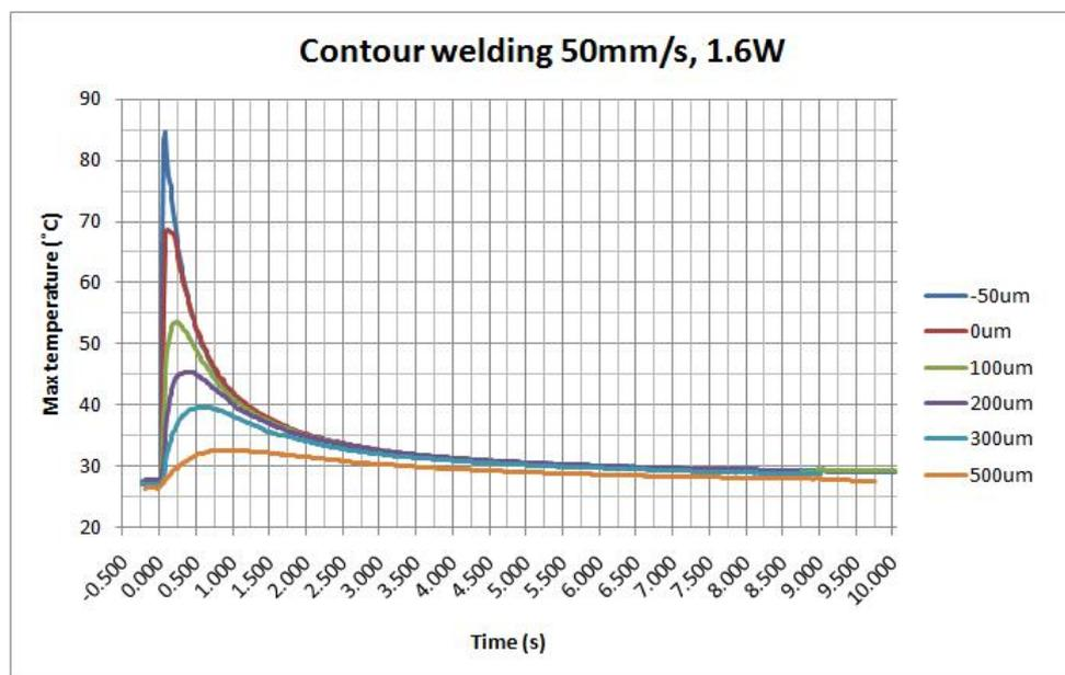
FIG. 7. The maximum channel temperatures during contour welding with 50 mm/s speed and 1.6 W laser power.
