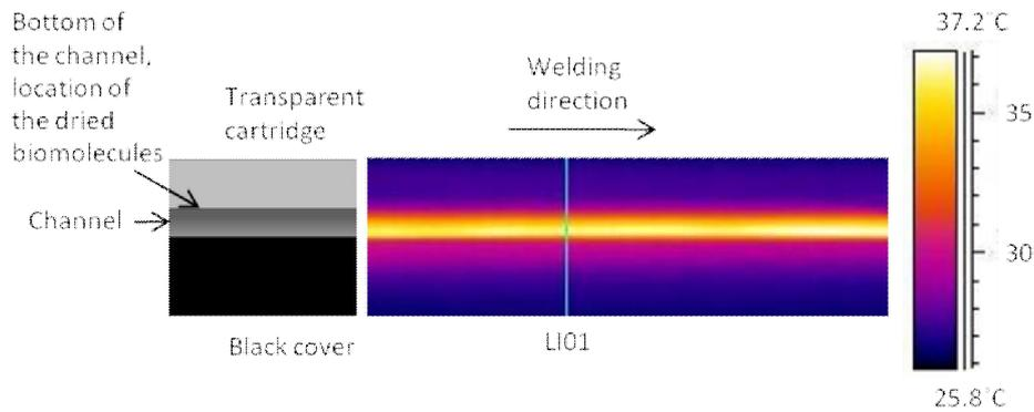
FIG. 9. Thermal image captured 3 seconds after the beam has passed the line LI01 using 100 µm welding distance between the seam and the channel wall. The temperature at the bottom of the channel is near to its maximum value.
