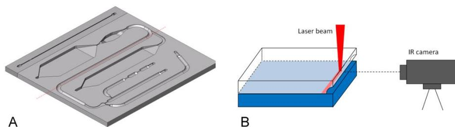
FIG. 5. (A) For the temperature measurements, the cartridges were cut in half. The dashed red line represents the cutting line. (B) A schematic drawing of the test arrangement for the channel temperature measurements.
