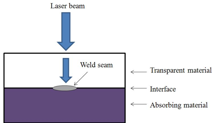
FIG. 1. The principle of laser transmission welding.
