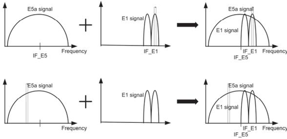
**Figure 7.** Illustration of signal superposition in the presence of narrowband interference
