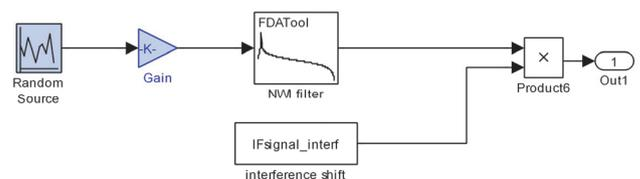
**Figure 3.** Interference generation
