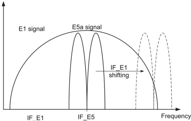
Figure 4. Illustration of IF shifting in simulation
