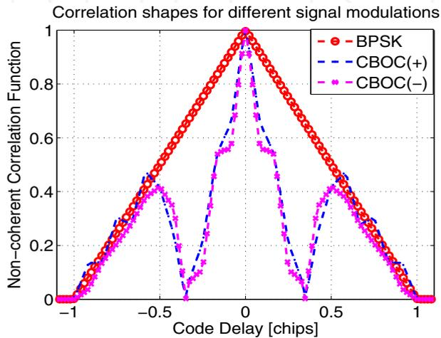
Fig. 2. Non-coherent correlation functions for different signal modulations.
