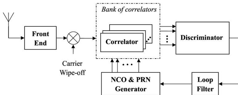
Fig. 5. Block diagram for multi-correlator based DLL implementation.
