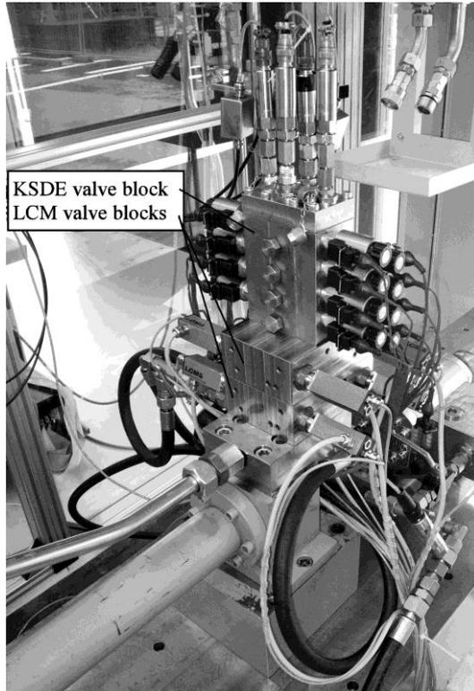
Figure 4. Valve blocks connected to the cylinder.
