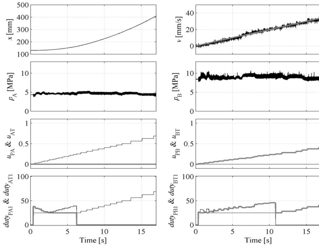
Figure 8. Slow ramp response to positive direction.
