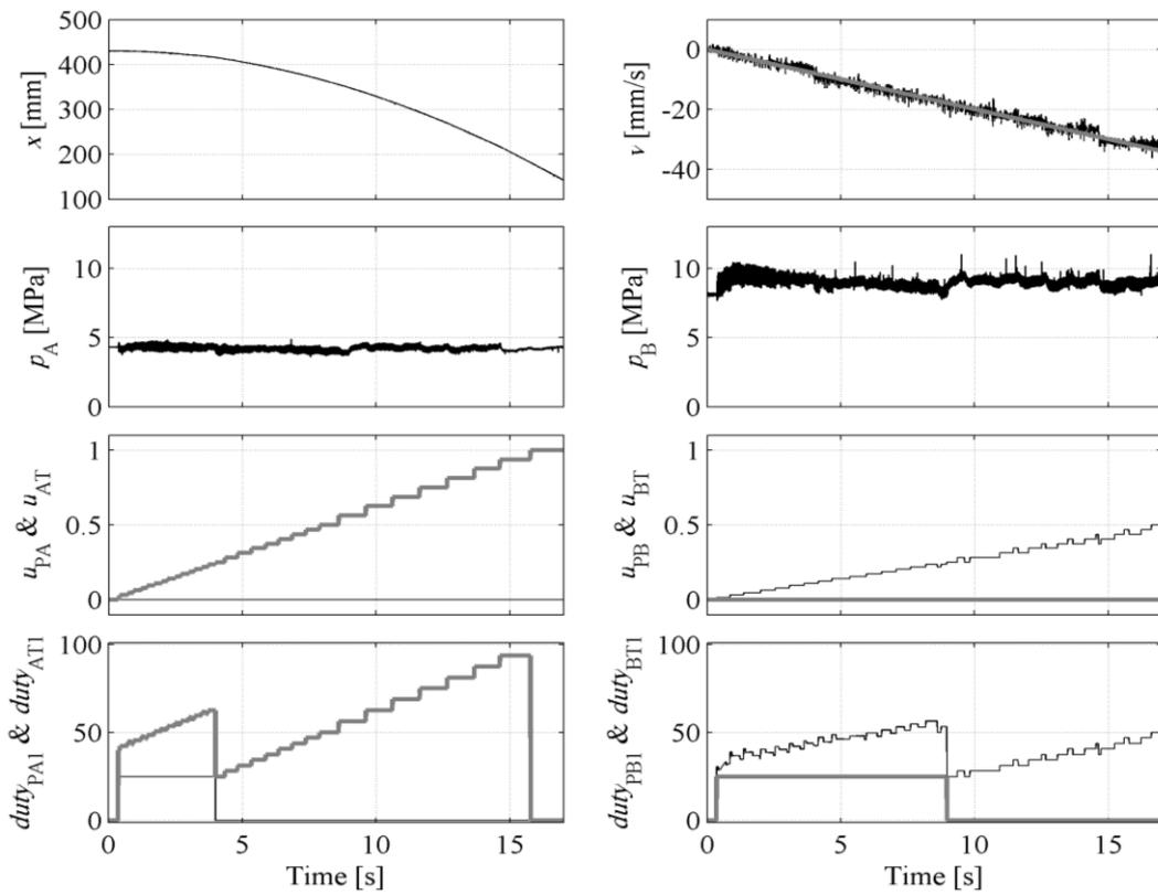
Figure 9. Slow ramp response to negative direction.
