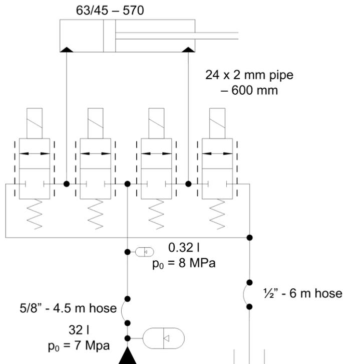
Figure 3. Hydraulic diagram of the test system
