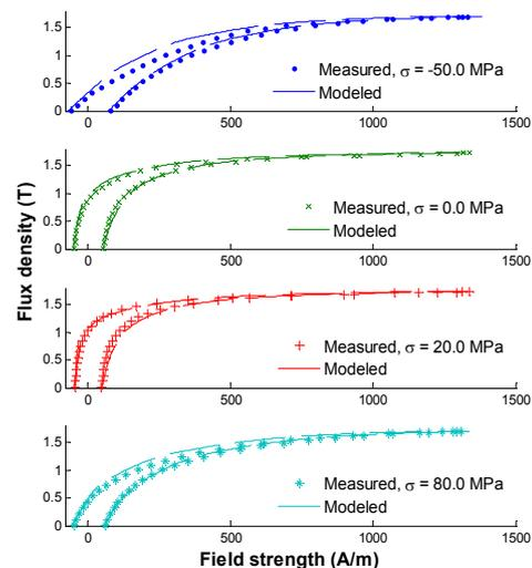
Fig. 3. Fitting the hysteresis model parameters  $k_0$ ,  $a$ ,  $b$ ,  $\alpha$  and  $c$  to the  $B$ - $H$  curve measurements at different compressive and tensile stresses
