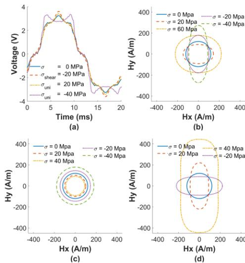
Fig. 4. Corresponding voltage waveforms in coils that are obtained from boundary conditions and locus of  $\mathbf{H}$  under different stress states and magnitudes (a) Evolution of the voltage waveforms under different stress states and magnitudes. (b), (c) and (d) Resulting  $\mathbf{H}$  locus under uniaxial, equibiaxial and pure shear stress states with different magnitudes.
