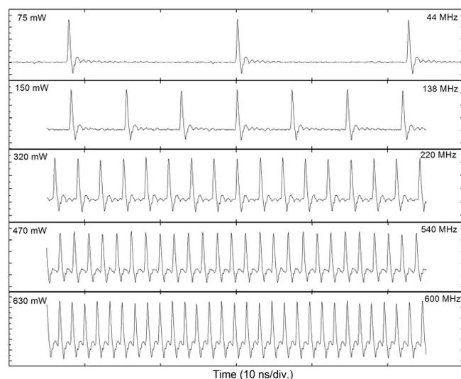
**Figure 6. The pulse trains for different pump powers.**
