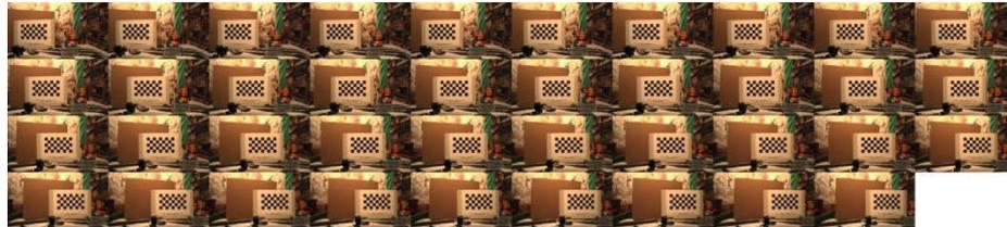
**Fig. 5.** Example of views taken with 11mm distance using LPS. Original data contain 400 views of size 1980x1080px taken with 1mm distance.
