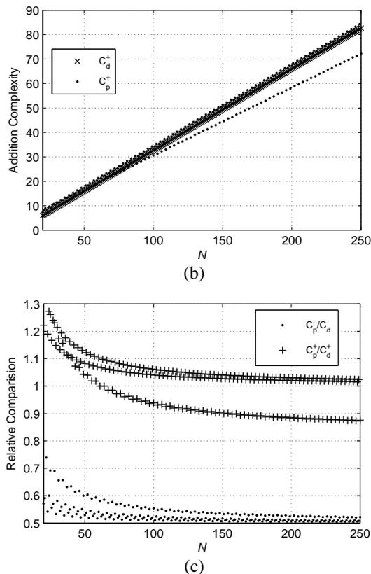
Figure 4. Implementation complexity for rational sampling rate converters by 3/5. Subindexes  $d$  and  $p$  stand for the polyphase and the proposed implementation, respectively. (a) Number of multiplications ( $C^*$ ) per output sample. (b) Number of additions ( $C^+$ ) per output sample. (c) Relative comparison between the proposed and polyphase implementation.
