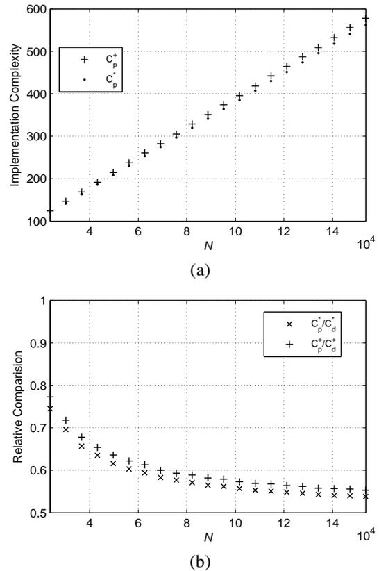
Figure 7. Implementation complexity for rational sampling rate converters by 147/160. Subindexes  $d$  and  $p$  stand for the polyphase and the proposed implementation, respectively. (a) Number of multiplications ( $C^*$ ) and additions ( $C^+$ ) per output sample. (b) Relative comparison between the proposed and polyphase implementation.
