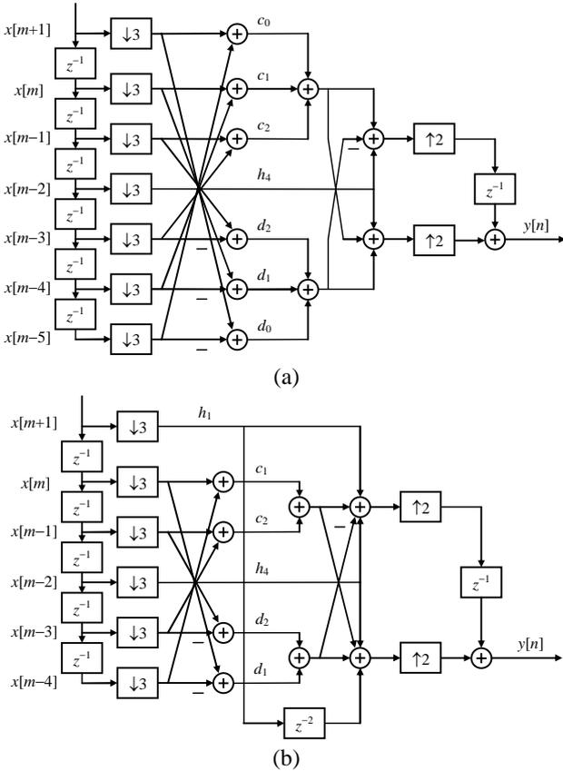
Figure 2. Implementation structure for a rational sampling rate converter by a factor of 2/3 using a linear-phase FIR filter of order  $N=11$ . (a) Proposed structure. (b) Alternative structure with additional delays.
