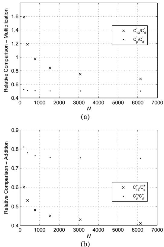
Figure 5. Comparison between the proposed implementation and the implementation described in [13] for rational sampling rate converters by 4/3. Subindexes  $p$ ,  $d$ , and 13 stand for the proposed implementation, polyphase implementation, and implementation proposed in [13], respectively. (a) Multiplication complexity. (b) Addition complexity.
