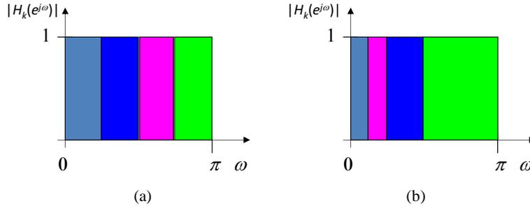
**Figure 3.** Some possible subband divisions for a four-channel filterbank. (a) Uniform filterbank for  $R = 4$ . (b) Non-uniform filterbank for  $R_0 = R_1 = 8, R_2 = 4, R_3 = 2$ .
