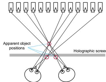
Figure 3. Light-field display architecture. Adapted from<sup>4</sup>
