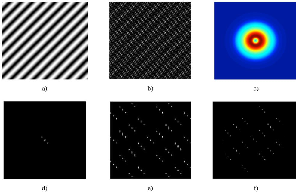
Figure 11. Intermediate stages of the pass/fail analysis: a) input signal, b) output signal, c) CSF weighting window, d) spectrum of the input signal, e) spectrum of the output signal, f) weighted spectrum of the output signal.
