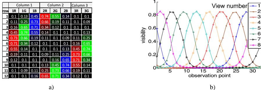
Figure 2. Angular visibility of multi-view display elements: a) visibility values for neighboring pixels as seen from the same observation direction, b) angular visibility functions of different views across the observation directions
