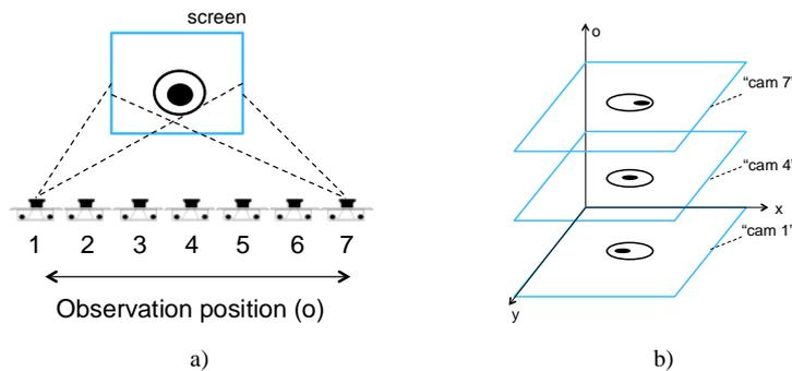
Figure 5. 3-dimensional ray description in  $(x, y, o)$  space: a) Multiple observations of the screen from different positions along the observation line, b) the same observations "stacked-up" in continuous  $(x, y, o)$  space
