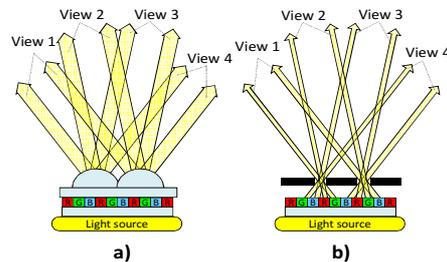
Figure 1. Optical separation in multi-view displays: a) using lenticular sheet, b) using parallax barrier
