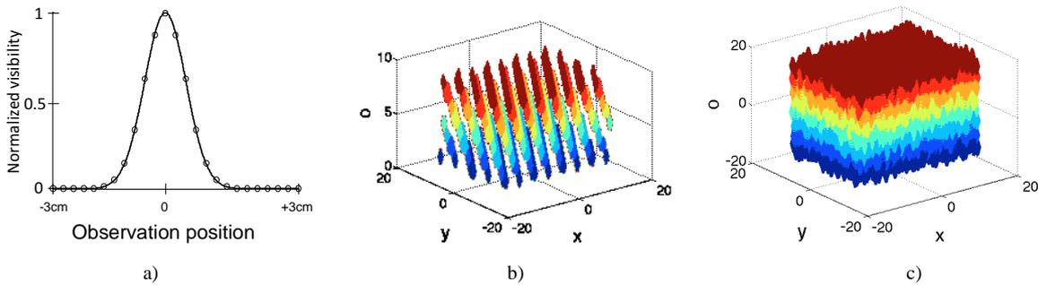
Figure 9. Angular visibility function: a) weighting coefficients as a function of the ( $o$ ) distance, b) multi-view display with the weighting coefficients applied, c) light-field display model with the weighting coefficients applied.
