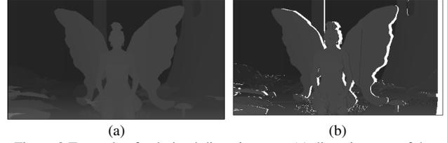
Figure 2 Example of a derived disparity map: (a) disparity map of the base view; (b) derived disparity map for a right side view, highlighting the occluded areas in white
