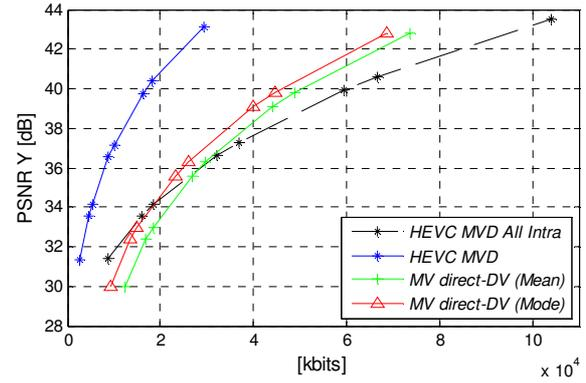
Figure 4 RD performance for the proposed *MV direct-DV* coding scheme
