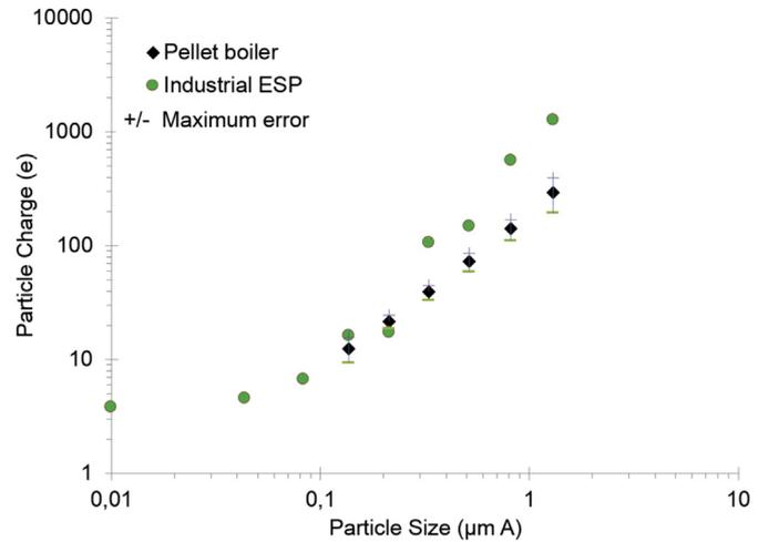
Fig. 7. Particle charge distribution achieved in the commercial pellet boiler tests. Two external GE chargers were used. Charge state measurement results from an industrial-scale ESP are also given for comparison.
