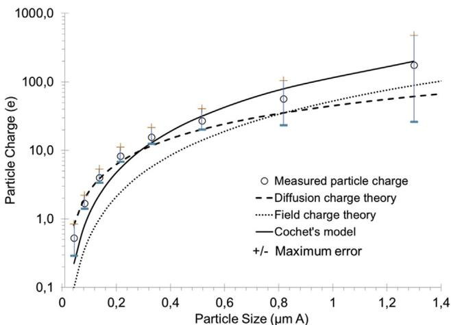
Fig. 6. Particle charge acquired with external GE charger. Fitted theoretical curves for diffusion charging, field charging and combined charging according to Cochet's model. Particle concentration of 530 mg/m<sup>3</sup>.
