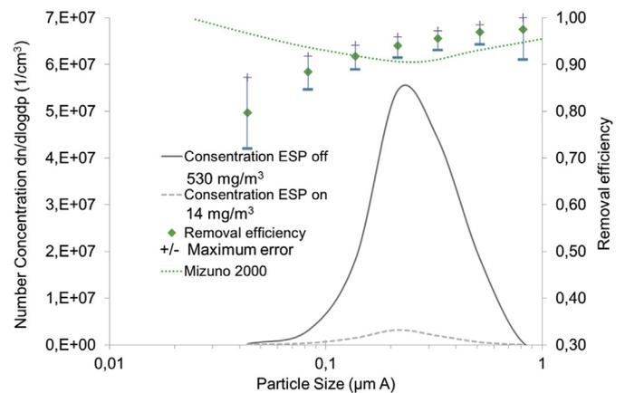
Fig. 8. Particle removal efficiency of the laboratory-scale parallel plate electrostatic collector. A single charger with an external ground electrode was used. ESP off = particle charging and ESP collection field off; ESP on = particle charging and ESP collection field on. Removal efficiency 97% from mass concentration. Removal efficiency 94% from particle number concentration. Result agree well with typical ESP removal efficiency. (Adaptation from Ref. [11]).
