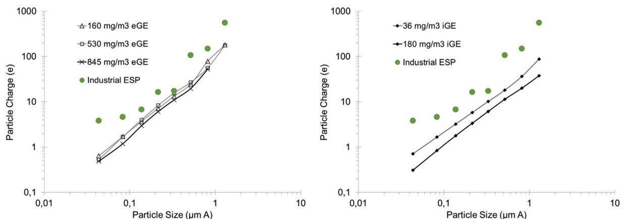
**Fig. 4.** Average particle charge distributions with different mass concentrations. Charger with integrated (iGE) and external (eGE) ground electrodes. Charge values below 1 elemental charge indicate that only some of the particles acquired a charge. For comparison charge distribution of an industrial ESP is also given.
