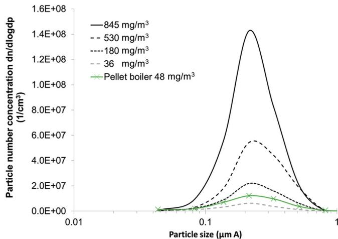
**Fig. 3.** Aerosol particle number distributions in laboratory measurements with different mass concentrations and the number distribution of a commercial pellet boiler. Particle size in aerodynamic diameter.
