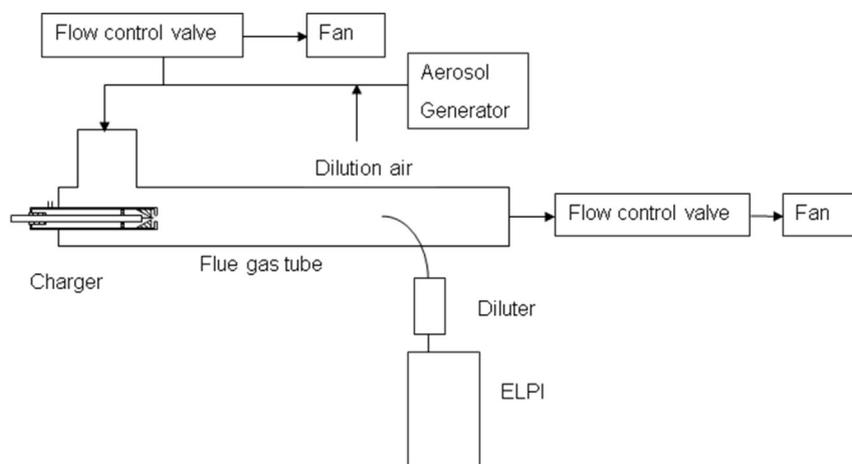
Fig. 2. Laboratory setup for the charging efficiency measurements.
