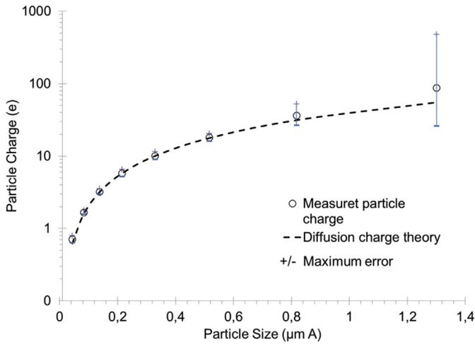
Fig. 5. Particle charge acquired with integrated GE charger. Fitted theoretical curve of diffusion charge. Particle concentration of 36 mg/m<sup>3</sup>.
