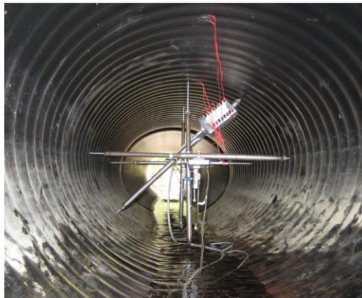
**Figure 2:** Installation of the displacement transducers used to monitor changes in the vertical and horizontal diameters of a plastic culvert.
