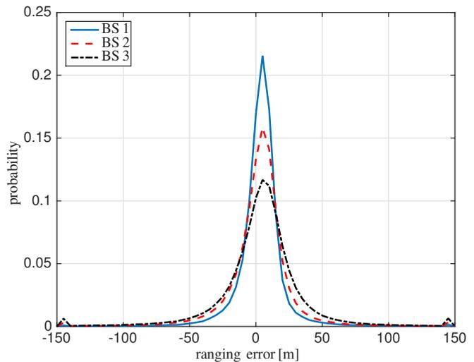
Fig. 7. Ranging error distribution for the three BSs in the EPA5 test.
