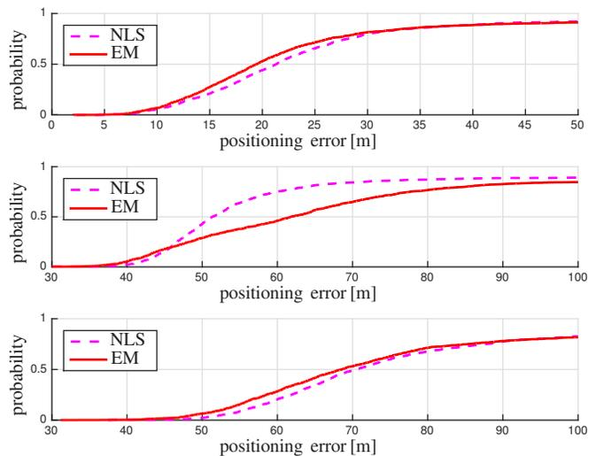
Fig. 4. Empirical CDFs of positioning errors for positioning tests of example topology. Upper plot shows the CDFs for the EPA5 channel model, plot in the middle shows CDFs for ETU70 channel model with TDE range  $[-0.5 T_s, 0.5 T_s]$ , and lower plot shows the CDFs for the ETU70 channel model with TDE range  $[-0.5 T_s, 6 T_s]$ .
