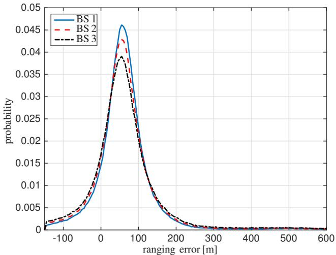
Fig. 9. Ranging error distribution for the three BSs in the ETU70 test with TDE range  $[-0.5T_s, 6T_s]$ . Ranging errors above 600 meters are not displayed.
