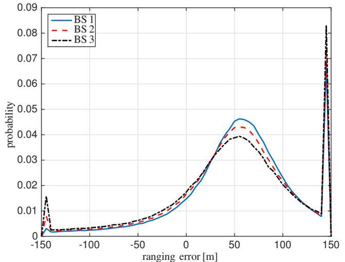
Fig. 8. Ranging error distribution for the three BSs in the ETU70 test with TDE range range  $[-0.5 T_s, 0.5 T_s]$ .
