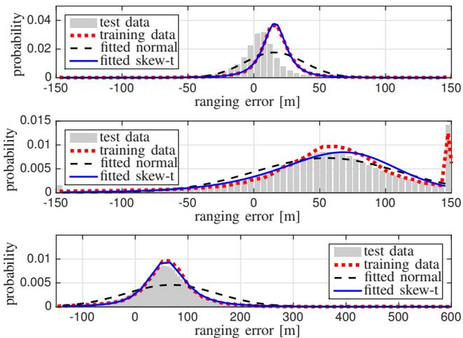
Fig. 5. Histogram of ranging errors in emulated LTE measurements for EPA5 (upper), and ETU70 channel with TDE range ranges  $[-0.5 T_s, 0.5 T_s]$  (middle) and  $[-0.5 T_s, 6 T_s]$  (lower; ranging errors above 600 meters are not displayed). Each figure contains in addition the empirical PDF of the training data and the PDFs of the normal and skew-t distribution fitted to the training data.
