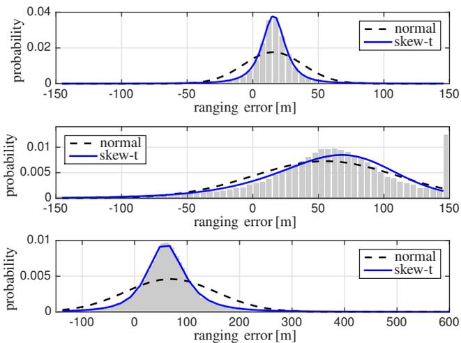
Fig. 3. Ranging error histograms with fitted normal and skew-t distributions for EPA5 channel model (upper), ETU70 channel model with TDE  $[-0.5T_s, 0.5T_s]$  (middle), and ETU70 channel model with TDE  $[-0.5T_s, 6T_s]$  (lower, errors above 600 meters are not displayed).
