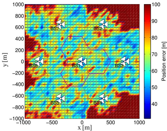
Fig. 10. Mean position error under ETU70 channel using EM algorithm, for which parameters were fitted to unrestricted data. Errors are limited to 150 meters. 65-degree sectors for each of the three antennas in each BS are denoted by triangles.
