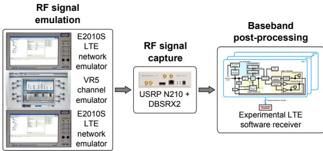
Fig. 2. LTE positioning testbed at ESA's Navigation Laboratory.
