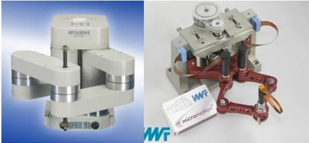
**Figure 2** On left, Mitsubishi RP robot [7] and on right, Parvus robot (image from [http://www.sfb516.tu-bs.de/english/t2/t2\\_en.html](http://www.sfb516.tu-bs.de/english/t2/t2_en.html)). Images are in different scales.
