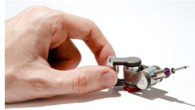
**Figure 8** Kleindiek Nanotechnik micromanipulator [13].
