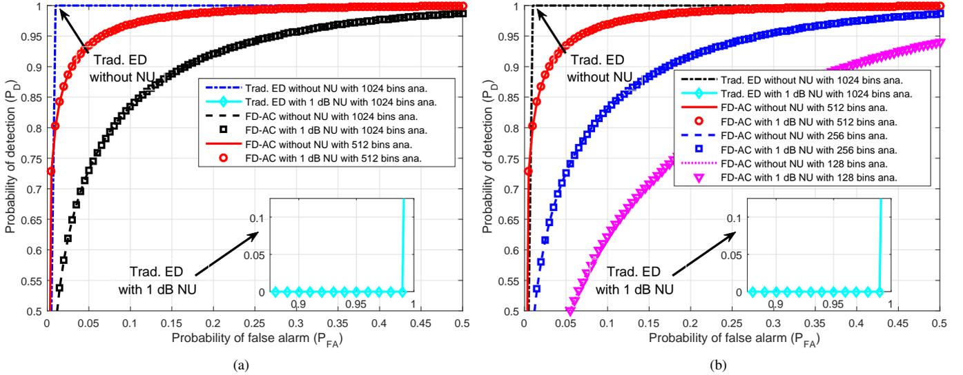
Figure 6: Receiver Operating Characteristics (ROC) curves of traditional ED and proposed FD-AC based sensing under  $-16$  dB SNR considering AWGN channel with/without NU with known time lag: (a) Magnitude test statistic, full-band sensing with 1024 bins, partial band sensing with 512 bins; (b) Magnitude test statistic, partial band sensing with 512 bins, 256 bins and 128 bins.
