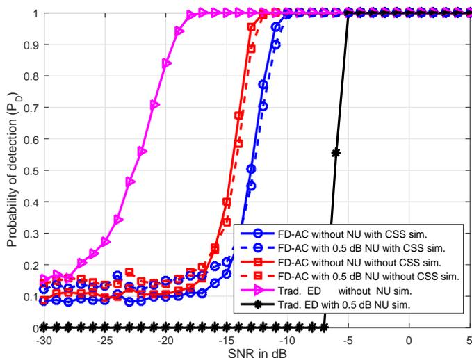
Figure 9: Detection probability of both traditional ED and proposed FD-AC based sensing in the case of unknown time lag without / with 0.5 dB NU and without / with compressed spectrum sensing under AWGN. The target  $P_{FA} = 0.1$  and  $K_{comp} = 242$ .
