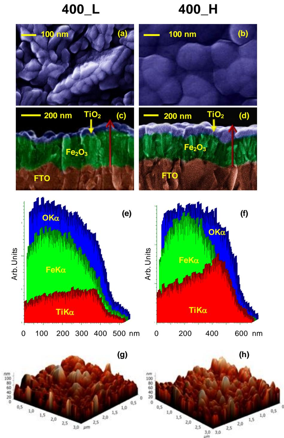
**Figure 1.** (a,b) Plane-view FE-SEM images, (c,d) cross-sectional FE-SEM images, (e,f) EDXS line-scan profiles recorded along the lines marked in cross-sectional views, and (g,h) AFM micrographs for  $\text{Fe}_2\text{O}_3$ - $\text{TiO}_2$  specimens. In (e) and (f), arrows mark the direction of abscissa increase.
