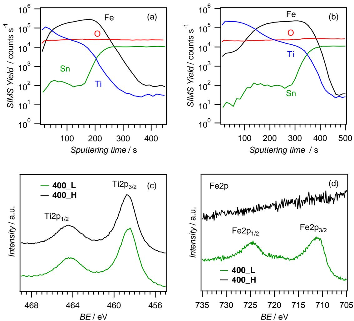
**Figure 2.** SIMS depth profiles for Fe<sub>2</sub>O<sub>3</sub>-TiO<sub>2</sub> deposits on FTO: (a) **400\_L**; (b) **400\_H**. (c) Ti2p, and (d) Fe2p XPS surface spectra for the same specimens.
