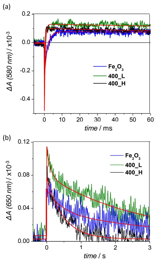
**Figure 5.** TAS decays for bare  $\text{Fe}_2\text{O}_3$  and  $\text{Fe}_2\text{O}_3\text{-TiO}_2$  samples on a millisecond (a) and a second (b) timescale. Red lines represent exponential fits of raw data.
