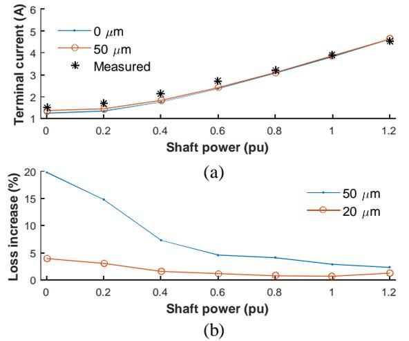
Figure 3: (a) Effect of the shrink-fitting on the terminal current of the PMSM and comparison to measurement results. (b) Increase in the total losses at two different shrink-fitting lengths compared to the unstressed case.
