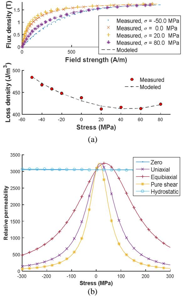
Figure 1: (a) Comparison of measured and modelled magnetization curves and hysteresis losses under uniaxial stresses and a parallel magnetic field. (b) Modelling results on the effect of different multiaxial stresses on the relative permeability at a constant flux-density of 1.5 T
