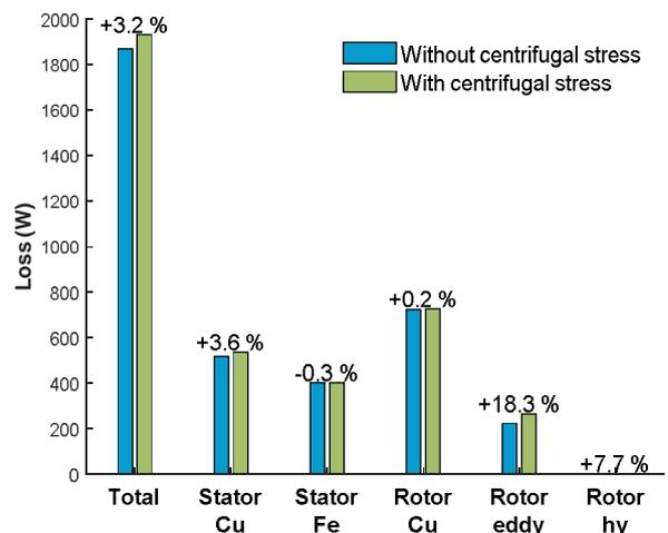
Figure 6: Segregation of the SRIM losses and their change due to the consideration of the centrifugal stress.
