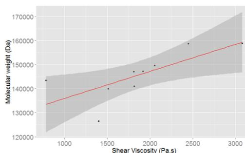
**Figure 1** Shear viscosity is plotted against Mw for all processing conditions. A line of best fit is plotted and a confidence interval of 0.95 is highlighted by the greyed region.
